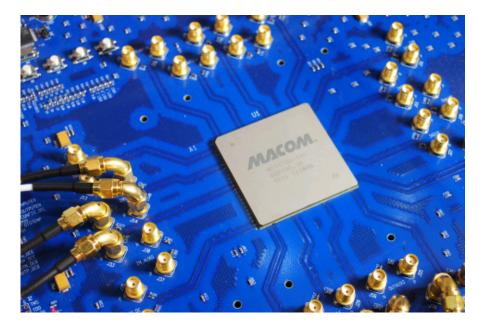
MACOM's M21170 crosspoint switch has been an integral component used in broadcast video routers and switchers around the world (Photo: Business Wire)
