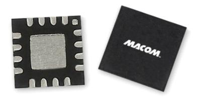
The MAAP-011232 features a typical gain of 23 dB and up 40% power added efficiency. The device can be operated between 5V to 9V and consumes less than 300 mA at maximum output power of 1 Watt. The MAAP-011232 device is fully matched while operating in the 100 MHz to 1GHz frequency range and can be tuned with input matched to perform up to 3 GHz. The device is offered in a 3mm 16 lead PQFN plastic package. (Photo: Business Wire)
