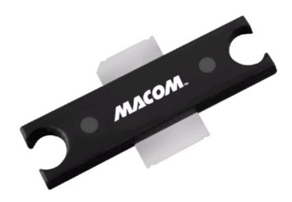
The MAGX-100027-100C0P supports CW, pulsed, and linear operation with output power levels up to 100 W (50 dBm). Featuring 50 V operation, this device offers CW operation of 18.3 dB gain at 2.45 GHz, and 70% drain efficiency. (Photo: Business Wire)
