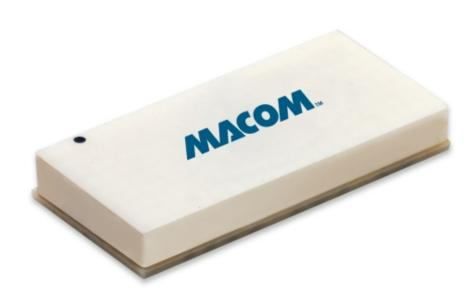
The device is a quad channel 32 Gbps modulator driver IC for 100G coherent transponders in CFP and CFP2 form factors. The device's low power dissipation, small size and high gain are key features that enable 100G coherent solutions in the size and power constrained pluggable form factors. (Photo: Business Wire)
