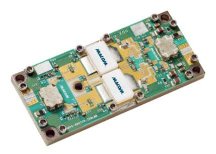
These new S-Band GaN power products provide integrated solutions which enable customers to accelerate time to market by leveraging commercial best practices for high-volume manufacturing, ensuring a host of additional benefits including improved assembly yield, lower component count, and reduced touch labor. (Photo: Business Wire)
