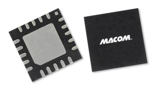
Packaged in a lead free 5mm x 5mm 20 lead PQFN the device offers a fully matched solution which can be used as a power amplifier stage or as a driver stage in high power pulsed applications. (Photo: Business Wire)
