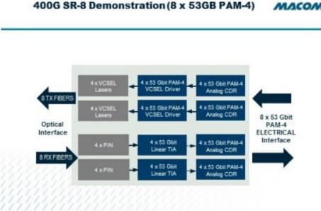
MACOM's fully analog chipset solution, featuring the MALD-38435 driver and MATA-38434 TIA along with MACOM's existing MASC-38040 and MAOM-38051/38053 CDR devices, offers customers that optimal high-performance, low power and low cost combination. By utilizing fully analog circuitry as opposed to digital signal processing, MACOM's solution delivers best in class low latency, especially critical for high performance computing applications. (Graphic: Business Wire)
