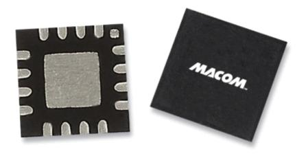
The single-ended, internally-matched MADT-011000 consumes 70  $\mu$ A from a 4.5 V supply, while the matched detector and reference diodes provide temperature compensation in differential operation. The MADT-011000 is offered in both a 3 mm 16-lead QFN package and in bare die format, with ESD protection for reliability and ease of handling. (Photo: Business Wire)
