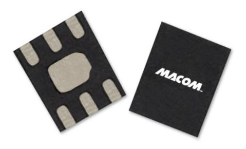
The integrated solution of the directional coupler and temperature compensated detector circuit enables customers to dramatically simplify their system designs and lower BOM costs while preserving valuable board space. (Graphic: Business Wire)
