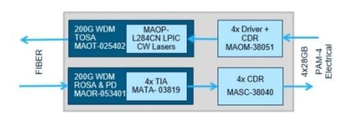
Introducing the industry's first complete chipset solution for 200G and 400G CWDM optical module providers servicing Cloud Data Center applications. This solution enables 200G modules at under 4.5W and 400G modules at under 9W total power consumption, thus delivering industry-leading power efficiency with a fully analog architecture that ensures extremely low latency and is poised to provide a lower cost option compared to DSP-based offerings. (Graphic: Business Wire)
